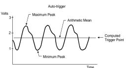
An automatic trigger mode is also available covering frequencies to 20 MHz with the minimum frequency selectable (as DC, 50 Hz, or 1 kHz) to optimize measurement speed.
